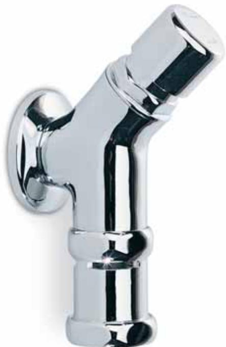
R 731 flussometro Ø 3/4" con dispositivo antisifonico incorporato erogazione per circa 6 sec. di 1,2 litri/secondo a 9 bar external pushbutton operated flushometer with built-in anti-syphon device 28/30 Ø outlet 1,2 l/sec. supplied for about 6 sec. at 3 bar
